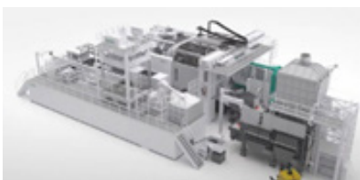
9.100 t GIGA-casting cell, BÜHLER
