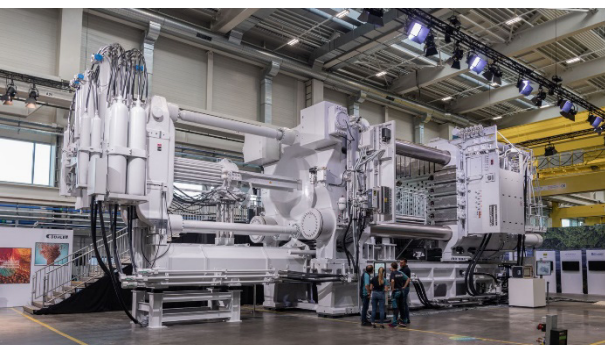
9.100 t GIGA-casting cell, BÜHLER
