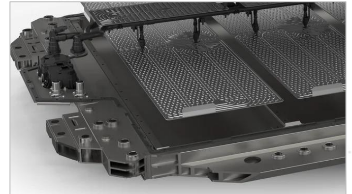
BMW i4 Battery Frame With Integrated Small Side Collision Rocker
