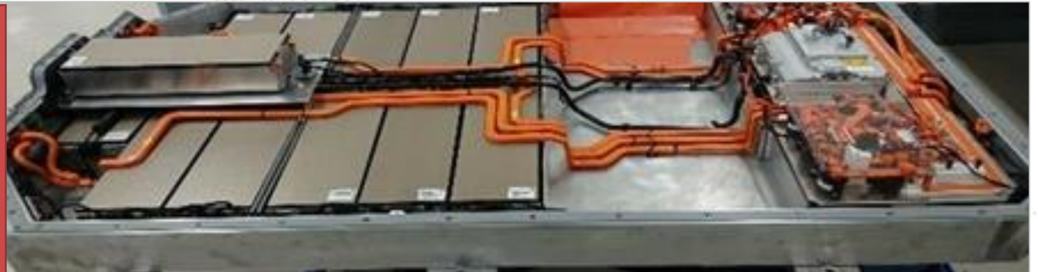
GEELY SEA LYNK&CO Zero EV HV Battery Frame Extruded AL
