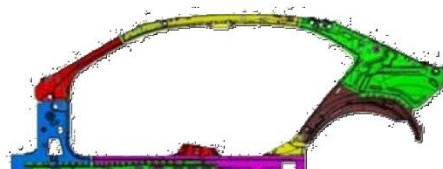
Sidewall inner (120 welds/car)
