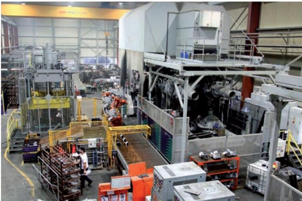
Die casting cell 3200t for 4-cavity production
