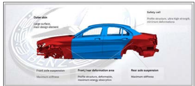
Figure 14. The lightweight material selection for the Mercedes-Benz C-class W205 hybrid body structure.
