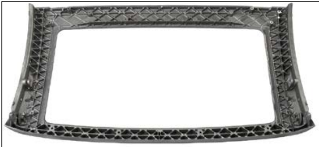
Figure 4. Example of a pre-series aluminum low pressure sand casting of the roof component for Daimler SL-class automobile supplied by Grunewald to specified high pressure die casting geometry, wall thickness and tolerances, and equivalent mechanical properties required by heat treatment and temper.
