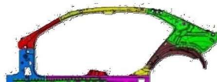
Sidewall inner (120 welds/car)
