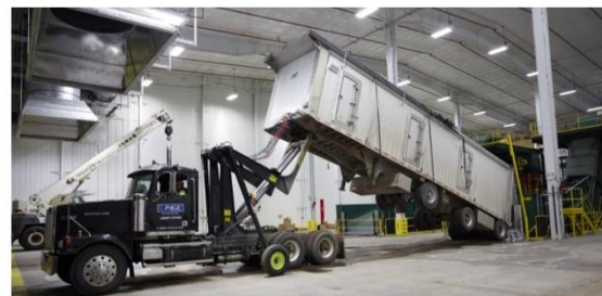
Specially designed trucks deliver scrap back from Ford's stamping plant to Novelis to be recycled
