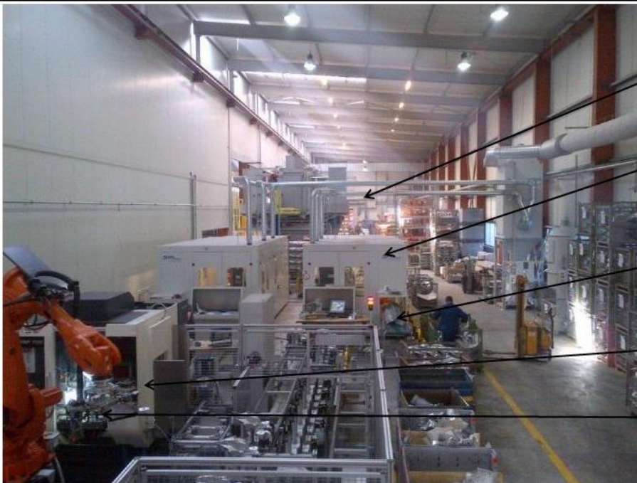
Heat treatment, grinding, measuring, machining and assembly process chain
