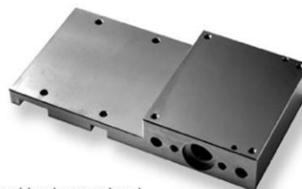
machined, ground and surface treated – the finished component
