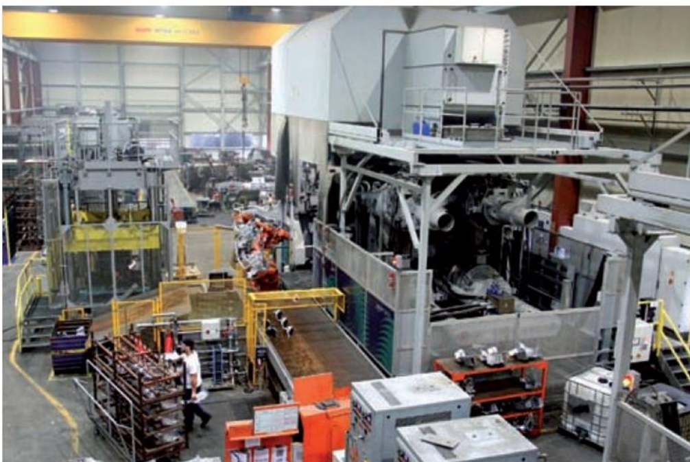
Die casting cell 3200t for 4-cavity production
