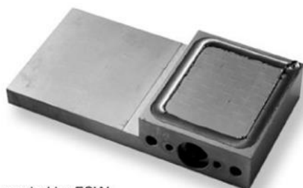
sealed by FSW in a CNC machine
