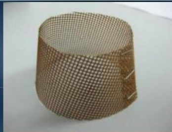
Fiberglass Screen Filter Which is Placed Between the Sprue (bottom mold half) and Sprue Spreader (upper mold half)
