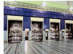
Four-stand Finishing Mill
