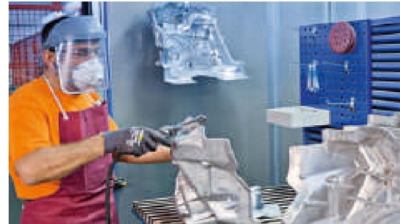
Manual cleaning of structural parts:
