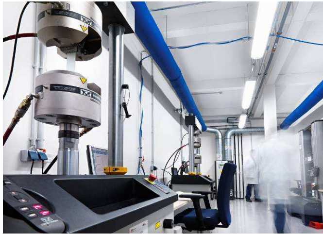
Static & dynamic (servo-hydraulic 100kN) test systems
