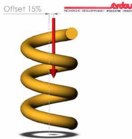
Glassfiber epoxy coil spring model, source: Sardou S.A.
