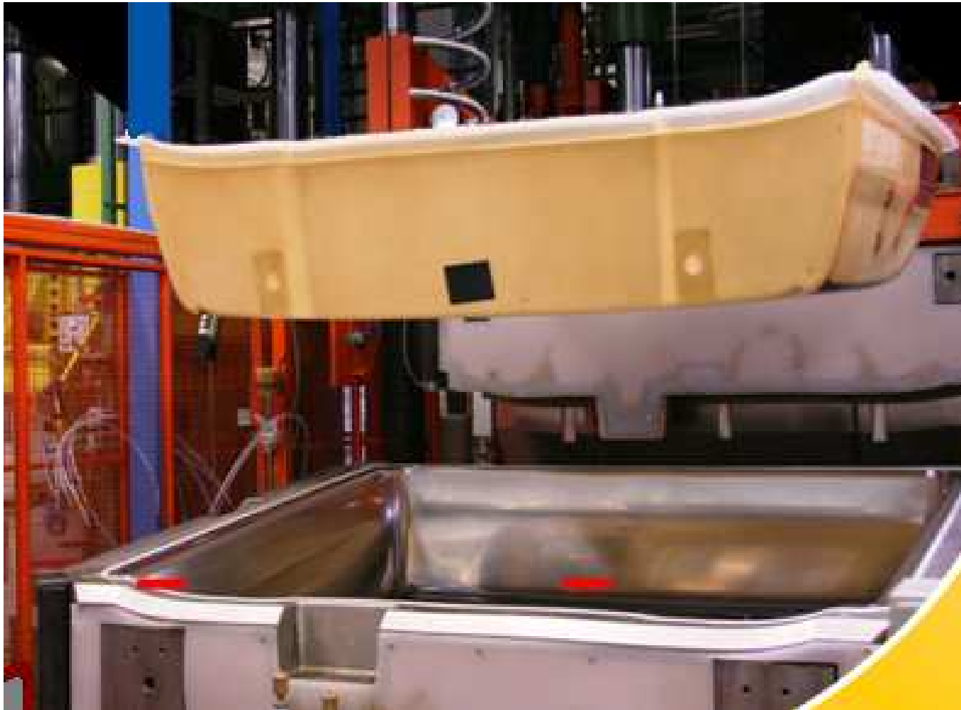
RTM mold and truck roof while demolding, source: Fritzmeier Composite
