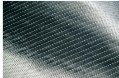
Multi-Axial Fabric utilizing our large tow carbon fiber optimized for RTM process
