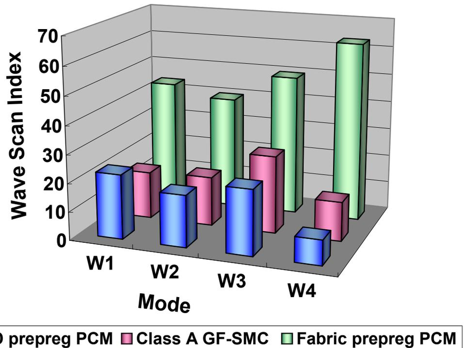
Wave scan index was measured by Wave Scan-T from BYK-Chemie
