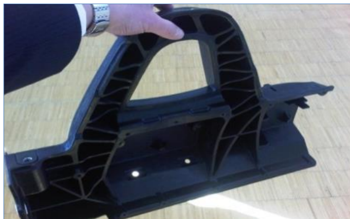
Mercedes SLK R172 roll over protection
