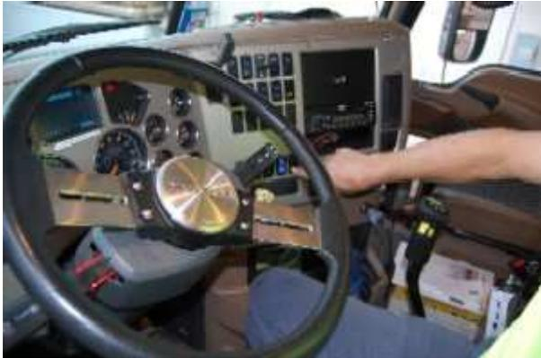
*[The blue switch Jimmie is pointing to started and stopped active regeneration of the DPF. With the SCR system on board, however, he almost never needs to press it now.]*
