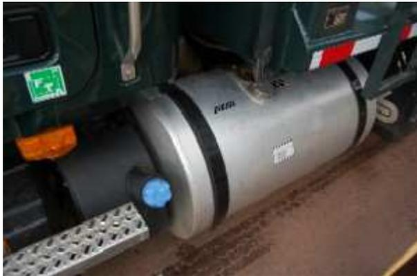
*[The tank with the baby blue cap on it holds the DEF. Mack also plans to use a D-shaped fuel tank for its 2010 production models, with the straight edge of the D facing out. That will offer more fuel capacity while leaving room behind the tank for cable bundles, hoses, etc.]*
